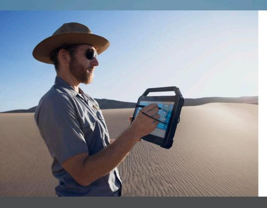
The Latitude 7220 Rugged Extreme Tablet features hot-swappable dual batteries, a 1000-nit outdoor-viewable screen, and is tested to withstand extreme temperatures: -20°F to 145°F.
