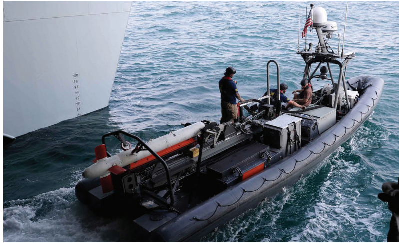
Peraton technicians assigned to Commander Fifth Fleet's mine warfare task force pilot a prototype Mine Countermeasures Unmanned Surface Vehicle out of RFA Mounts Bay's well deck during a US-UK bilateral exercise. Photo source: U.S. Navy
